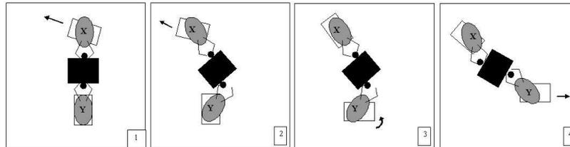
Figure 3: 1) robot (X) is pulling and the other (Y) is listening; 2) The object rotates, causing a rotation of the head of (Y) in a wrong direction; 3) (X) stops its unsuccessful retrieval while the second (Y) rotates to its right; 4) (Y) is pulling causing a rotation of the object and of the head of (X) in a wrong direction, as in 2) for (Y)
