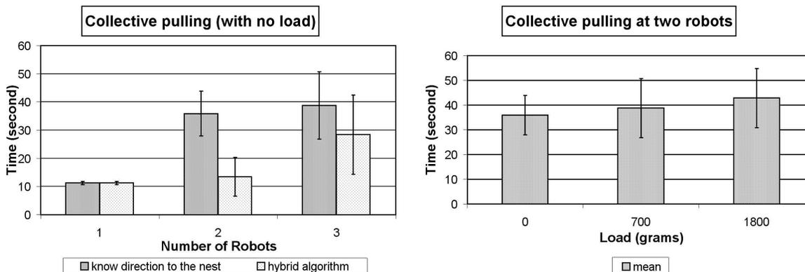
Figure 4: 1) mean retrieval time in function of the number of robots on 10 trials with 2 different algorithms; 2) mean retrieval time at two robots in function of the load (on 10 trials)
