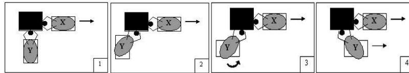
Figure 2: 1) (X) is pulling and robot(Y) is listening; 2) The head from the listening robot (Y) rotates right due to the force exerted by the pulling robot(X); 3) The listening robot (Y) rotates right; 4) Both robots are pulling in the same direction
